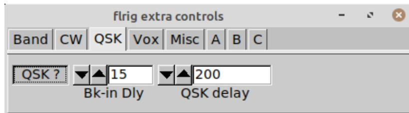
The QSK tab allows you to select Semi-breakin or Full-breakin with the QSK button. Bk-in Dly sets the time delay during Semi-breakin operation so the rig does not return to receive while keying. QSK delay does the same thing during Full-breakin operation.
