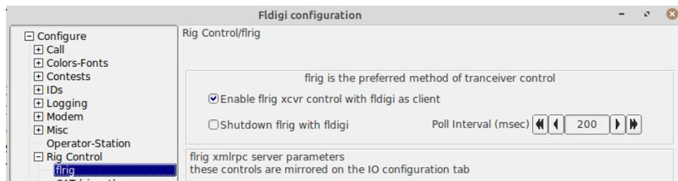
Deselect all other rig control methods and enable fldigi as an flrig client. Xmlrpc is used via a local socket device for the two programs to communicate. flrig acts as the server and fldigi the client. There is no requirement for start / stop ordering of the programs.
