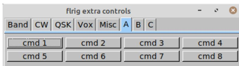
The A, B, and C tabs are 3 sets of 16 entries that can be CAT commands to perform functions that flrig does not have coded for your radio. Things like setting audio output level or any other functions that can be CAT controlled. Entries are setup via the flrig Config/Setup/Commands tab. See Chapter 10, User-Defined Commands, in this document.
