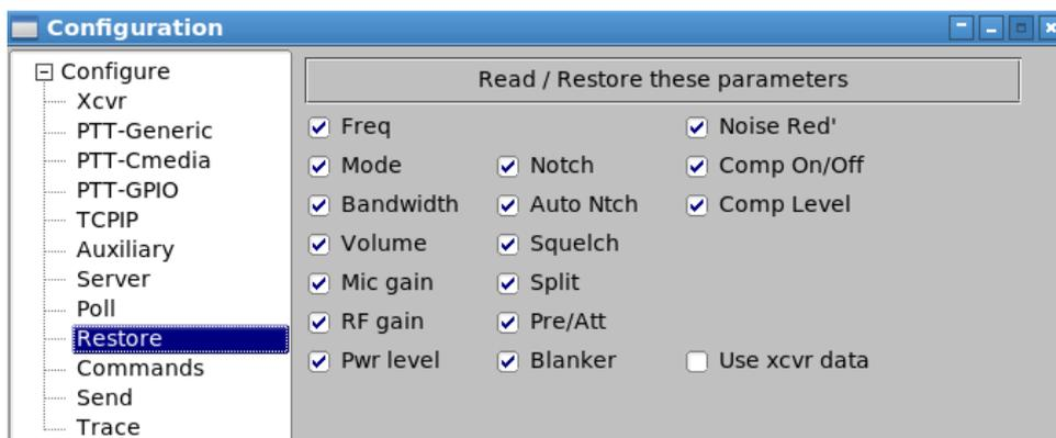
and choose whether you want flrig to save and restore all the radio's parameters on startup and exit or whether you want it to open with the same settings as the rig is currently using. If Use xcvr data is checked flrig will start up with the same settings as the rig currently is using.
