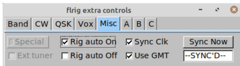
For those rigs with CAT controlled Power On/Off available set it as desired. Auto-on activates when flrig is first started. Auto-off activates as flrig shuts down. If the computer has CAT controlled time setting available flrig can set the rig's internal clock to the computer's time/date. This happens on the exact minute so you will see it showing the time until it has synchronized.
