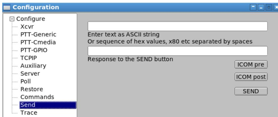
Figure 12.2 I/O Ports - Sending
