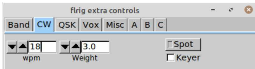
The CW tab is pretty well self explanatory. Set the WPM as desired. Weight refers to the ratio of Dit to Dash, but is not available on all rigs. What other controls are visible will depend on the rig being used.
