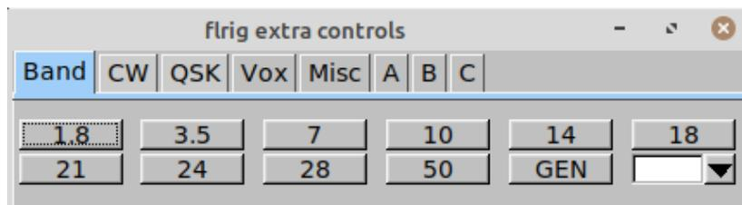
Left-click on a Band button to QSY to that band. Typically this will apply the settings saved in the top register in your rig's Band Stacking Registers for that band, if your rig supports BSR. This should provide similar functionality to physically pressing the rig's Band button. For example, on an Icom IC-7610, this will recall the frequency, mode, filter selection, and if FM mode, the tone frequencies last used on the selected band.
