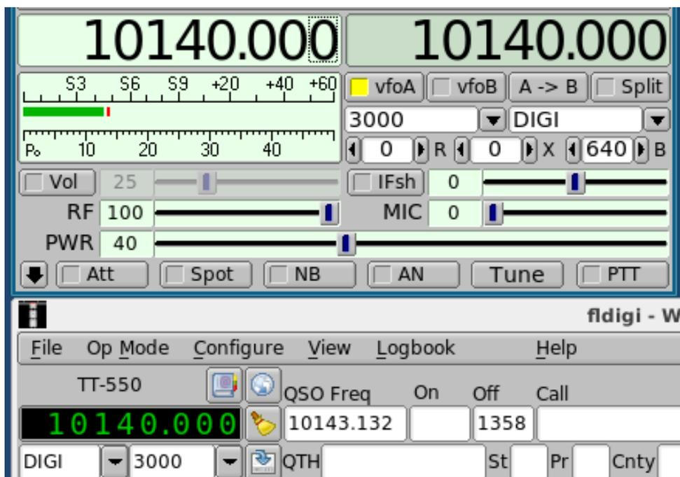
Once that is done fldigi should communicate with flrig and changes such as frequency or bandwidth in flrig or fldigi should be reflected in the other. If the lower box is checked then flrig will send fldigi audio to the radio when the PTT button is clicked otherwise PTT will just key the rig with no power out. Click Save at the bottom of the page.
