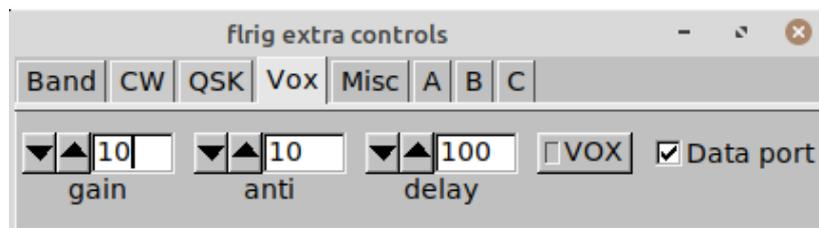
**Gain** refers to the sensitivity to your voice causing it to switch to transmit.
